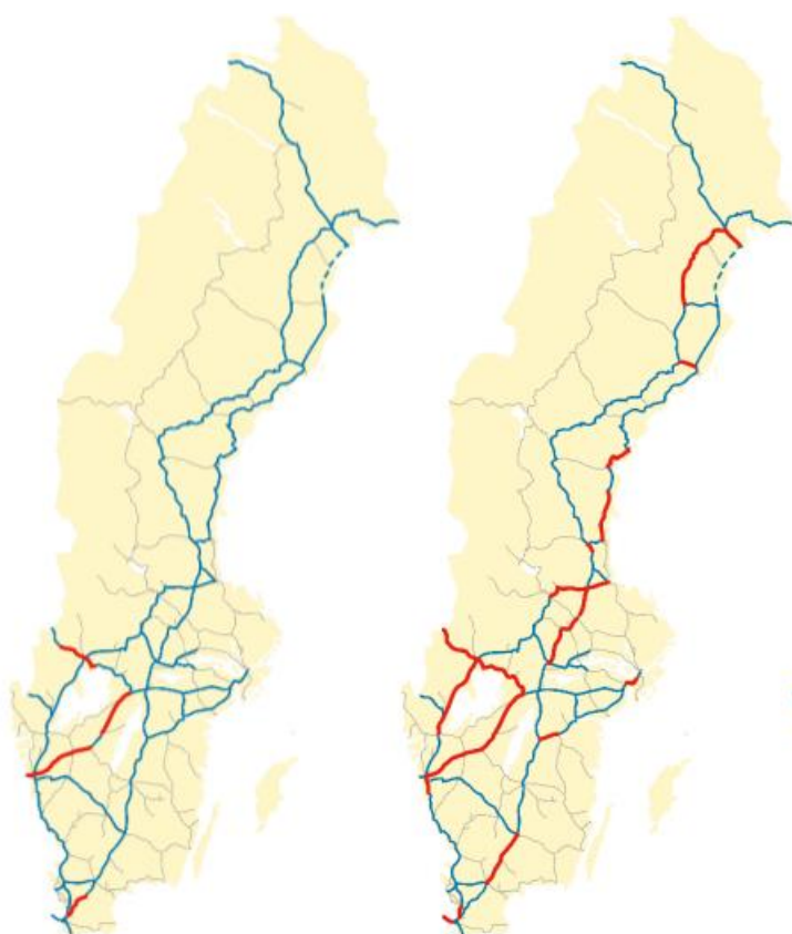
Figure 42. Rail capacity in Sweden. Red indicates a significant shortage of capacity for freight transport measured over the day (capacity utilization >80% and \geq 20 freight trains per day). The map on the left is 2019 and the right is with investments according to the national transport plan 2018-2029 with the base forecast for 2040. Source: Trafikverket 2021b p.21.
